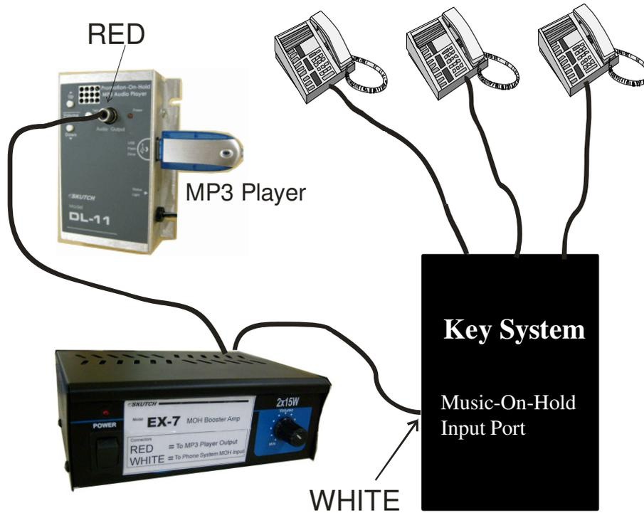
1- Connect the RED RCA Plug from the EX-7 to the output of the MP3 Player or Audio Source. This is the “INPUT”
