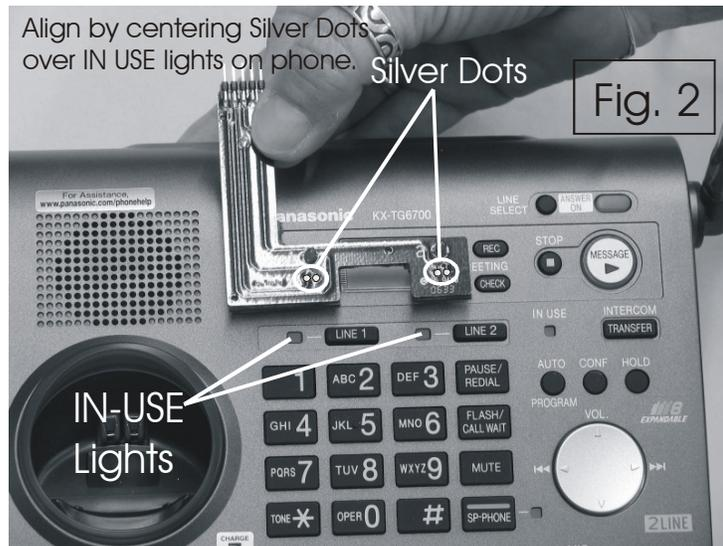
5- Make sure that the surface area of the base phone, where the sensor board is to be mounted, is clean and free of all dust and oil film. Locate the CK-1P4 "SENSOR BOARD", peel off the green/white protector papers from the bottom of the sensor board, and carefully place it OVER the LINE 1 and LINE 2 lights on the Panasonic base set as shown in Fig. 2 and Fig. 3. Make sure that you align the SILVER DOTS on the Sensor Board, directly over the IN-USE lights on the phone.
