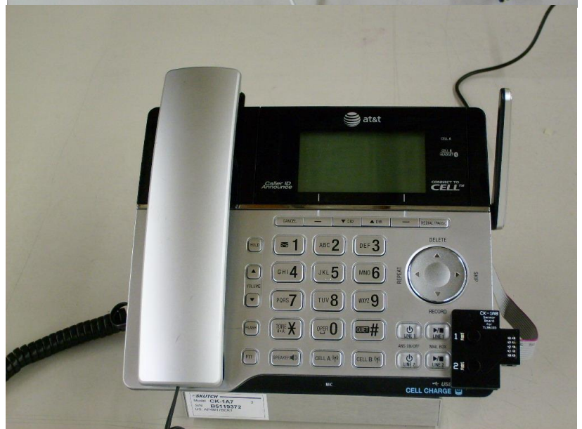
CK-1A8 Installed on TL86103
