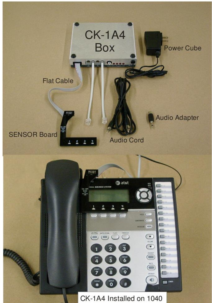
1- Position the CK-1A4 box under the telephone with the jacks facing towards the back of the phone. (See Fig. 3).
