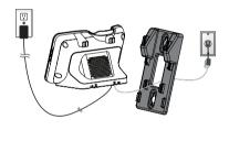
3. Position the lower portion grooves on the telephone base to the lower portion tabs (marked B) on the wall mount bracket. Make sure the upper portion grooves of the telephone base are above the upper portion tabs (marked A) on the wall mount bracket. Push the telephone base down until it clicks securely in place.
