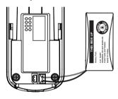
Place the battery with the label THIS SIDE UP facing up and the wires inside the battery compartment.
