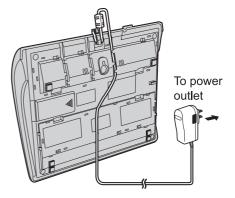
**3** Dress the telephone line cord as shown. Tuck the telephone line cord inside the wall mounting adaptor, then push it in the direction of the arrows (① and ②).
