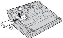
2 Match the polarity and snap the battery to the battery snap as shown.
