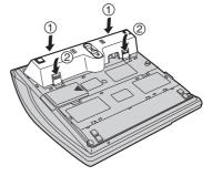
• To attach the wall mounting adaptor, push it in the direction of the arrows (① and ②) as shown.
