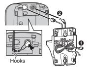
Insert the hooks on the wall mounting adaptor into holes and
