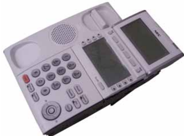
Figure 5-66 8LKD (LD)-L UNIT Installed
