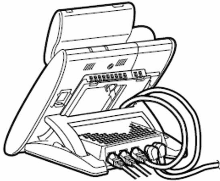
Figure 9-86 GBA-L UNIT Installed
