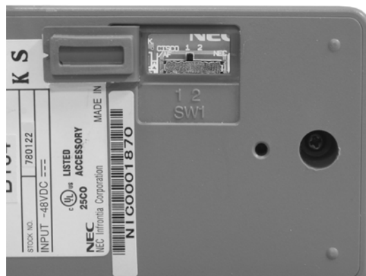
Figure 9-46 In-Line Power Adapter Switch Settings
