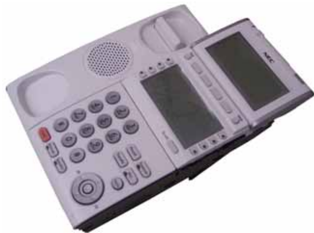
Figure 5-72 8LKI (LD)-L UNIT Installed
