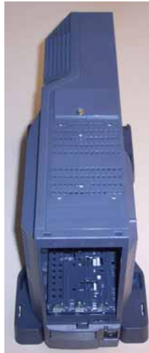
Figure 3-92 Stand Mount Brackets Installed
