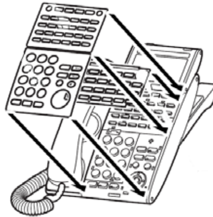
Figure 9-71 Install Plastic Panels
