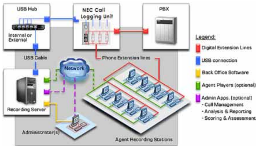
Figure 9-35 Digital Call Logging Unit Connection Configuration
