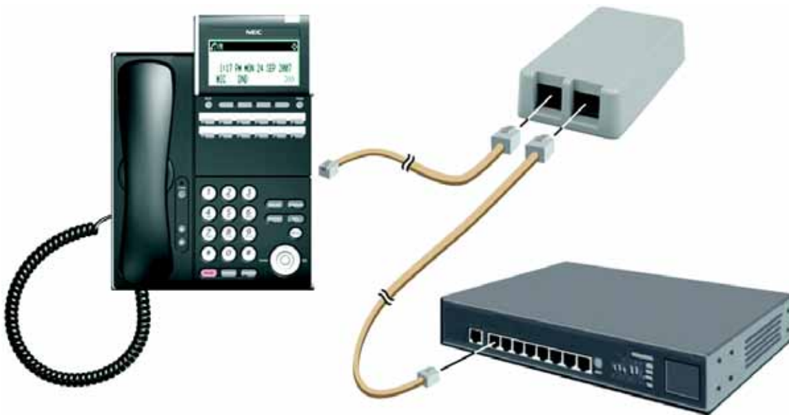
Figure 9-47 NEC Terminal Connection to an IEEE 802.3af PoE Switch
