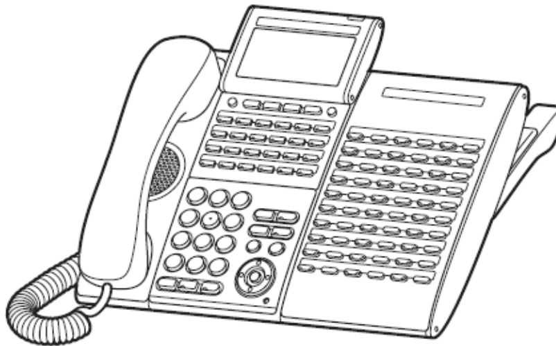
Figure 5-81 DCL-60-1 CONSOLE Installed
