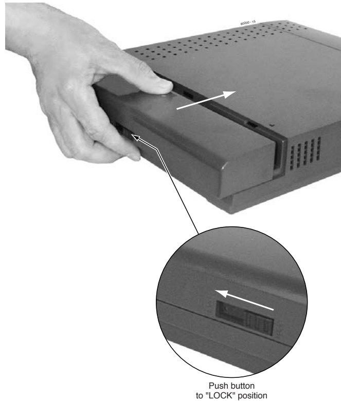
Figure 3-5: Reinstalling the Cover
