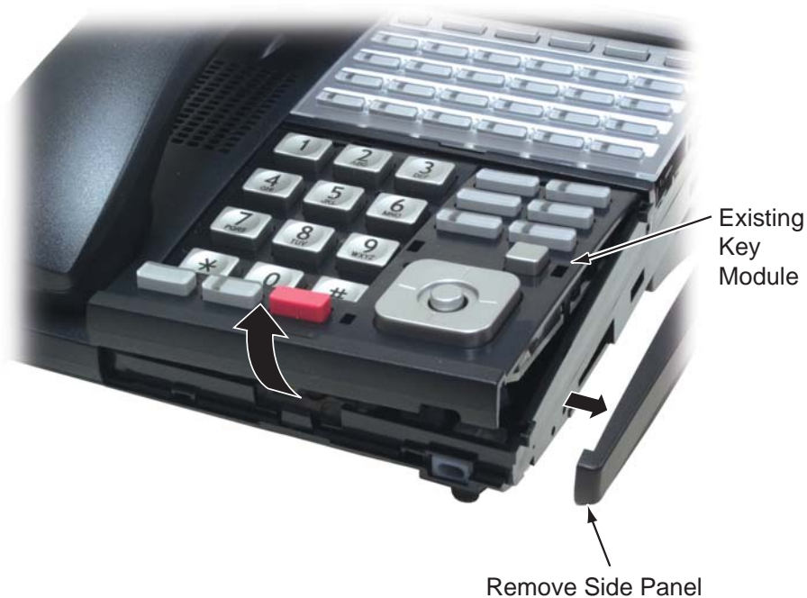
Figure 4-10: REMOVE EXISTING KEY MODULE AND SIDE PANEL
