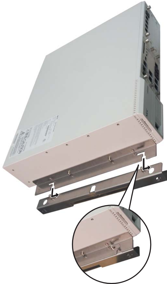
Figure 1-63: HOOK THE CHASSIS-A ONTO THE WALL MOUNT BRACKETS
