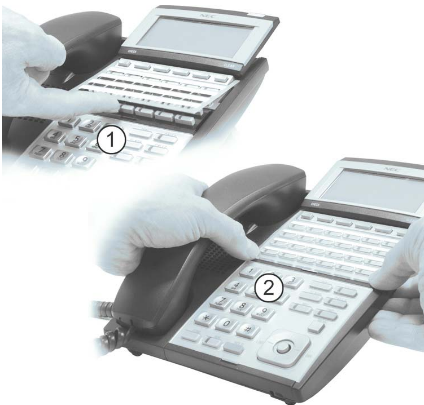
Figure 4-40: REPLACING THE FACEPLATE
