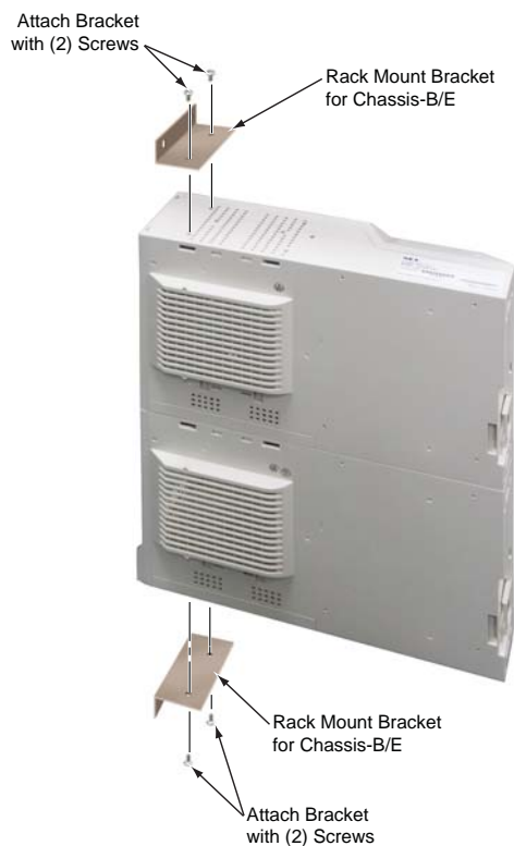
Figure 1-91: ATTACH RACK MOUNT BRACKETS TO CHASSIS-B/E
