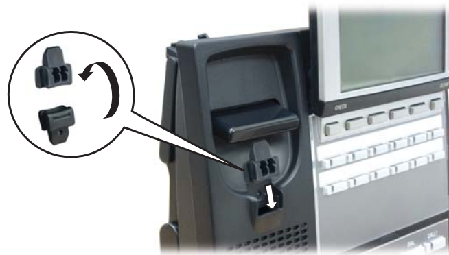
Figure 4-47: INSTALLING THE HOOKSWITCH HANGER
