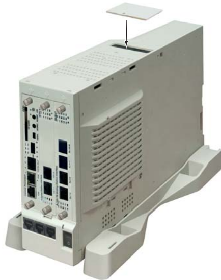
Figure 1-69: ATTACH THE BACKBOARD CONNECTOR COVER
