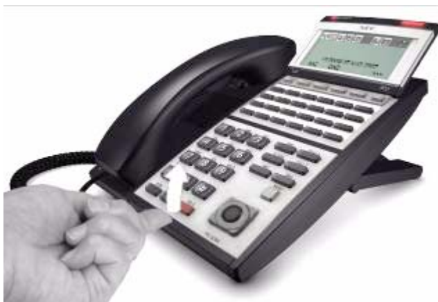
Figure 4-39: REMOVING THE FACEPLATE
