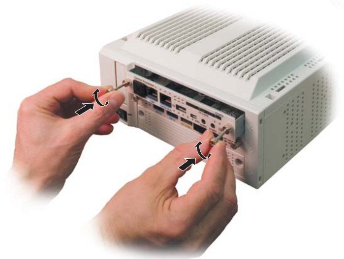
Figure 2-7: TIGHTEN THUMB SCREWS
