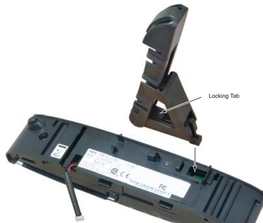
Figure 4-44: ATTACHING THE TERMINAL LEG(S)
