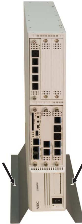
Figure 1-76: FLOOR MOUNTING 1 CHASSIS-A
