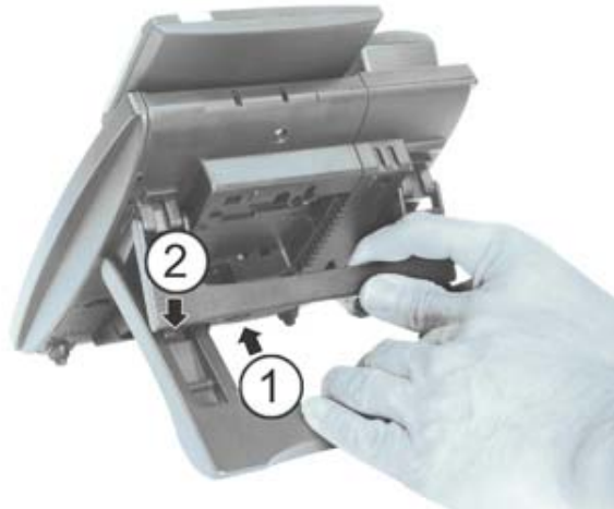
Figure 4-42: INCREASING THE TERMINAL HEIGHT
