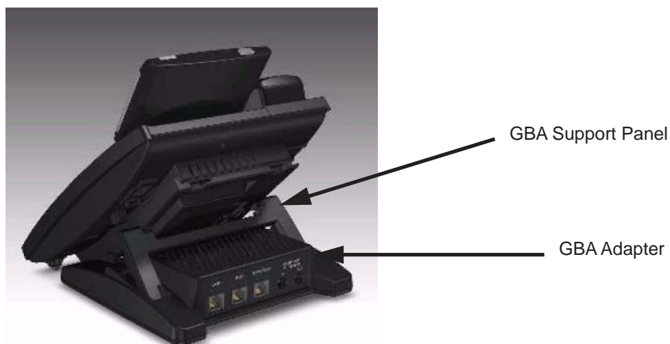
Figure 4-26: INSTALLED GIGABIT ADAPTER
