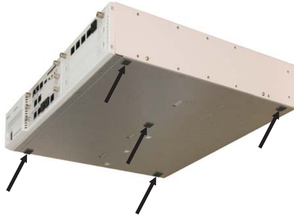
Figure 1-77: ADD RUBBER FEET FOR MULTI-CHASSIS INSTALLATIONS
