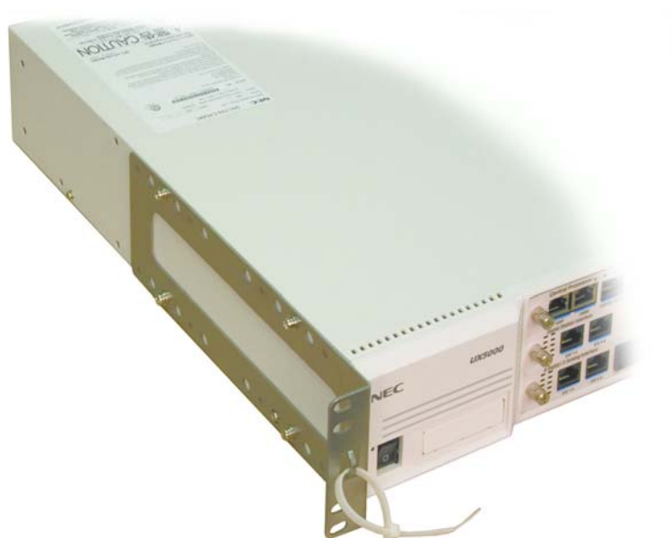
Figure 1-92: ATTACH RACK MOUNT BRACKETS TO CHASSIS-A
