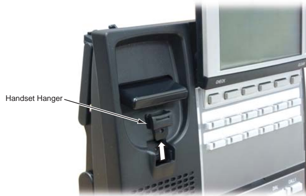
Figure 4-46: REMOVING THE HOOKSWITCH HANGER
