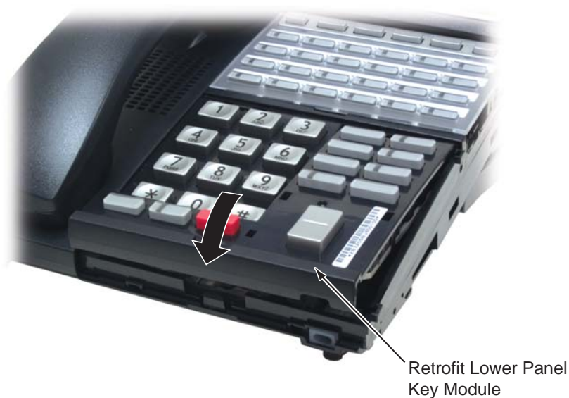
Figure 4-12: PRESS RETROFIT LOWER PANEL INTO PLACE
