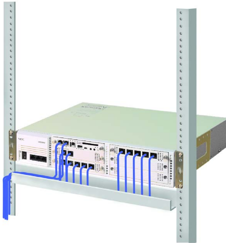
Figure 1-90: 19" CHASSIS-A RACK MOUNT INSTALLATION
