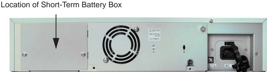
Figure 1-17: SHORT-TERM BATTERY BOX LOCATION ON 19" CHASSIS-A
