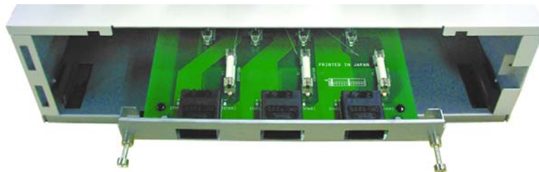
Figure 1-44: REMOVE FUSE BOARD
