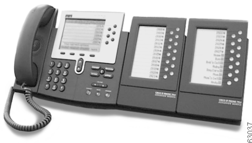
Figure 6-1 Cisco IP Phone 7960 with Two Expansion Modules
