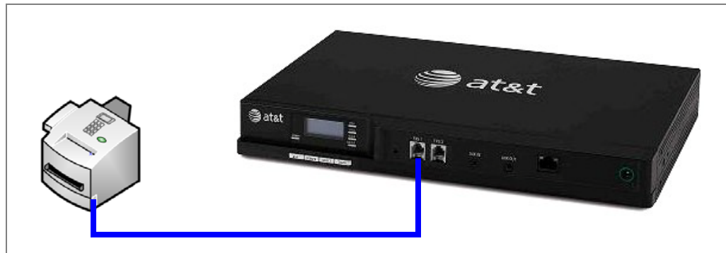
Figure 10. Fax Machine Connected to FXS Port
