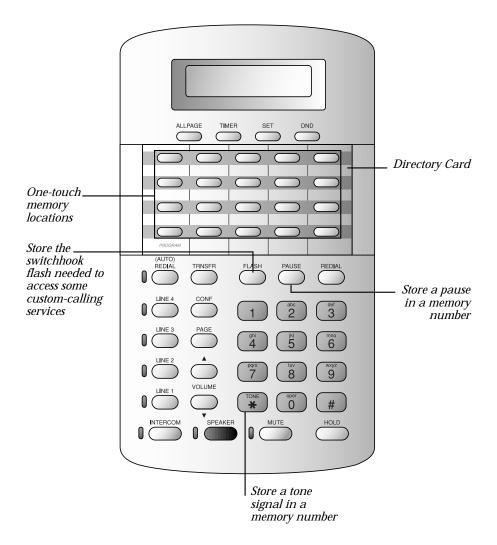
This telephone has 19 memory locations. Each location can store up to 16 digits. Dial numbers stored in memory locations by lifting the handset (or pressing <u>SPEAKER</u>) and pressing the button for the location.
