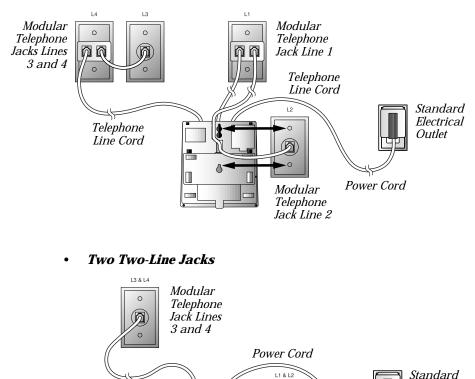
**NOTE:** If you have three modular telephone jacks, mount the phone onto a jack without a wall-mounting adapter. If you have four modular telephone jacks, mount the phone onto a jack without a wall-mounting adapter.
