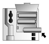
3 Turn the base, as shown, and attach it to the bottom of the phone.
